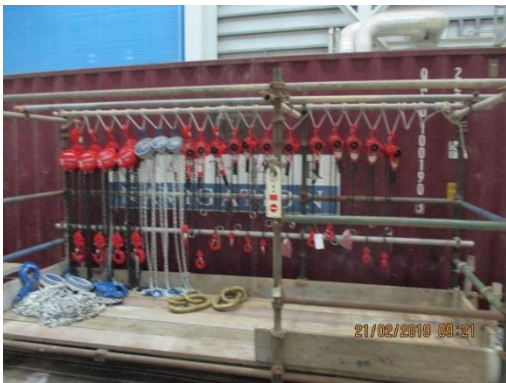
Lifting gears storage (hanged safely – Chain block)
